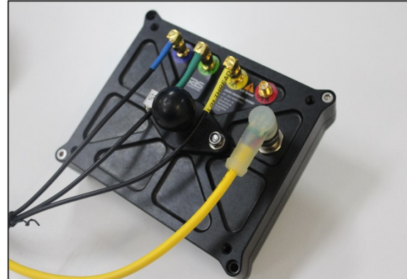
Rear panel of the unit, with all aerial and power leads connected.
