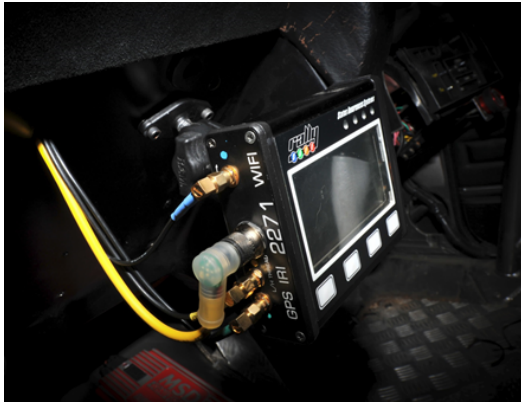
A standard installation. Note: unit and aerial placed in clear and unobstructed view.
